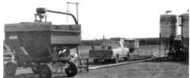
FIGURE 11. Increased Discharge Pipe Length.
