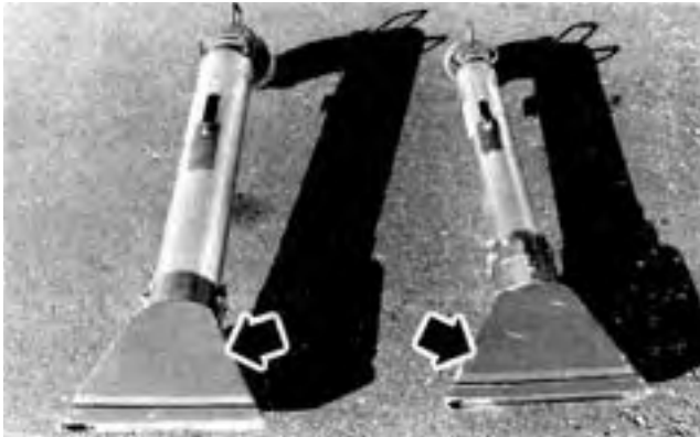
FIGURE 4. Flared Ends on Intake Nozzles.
