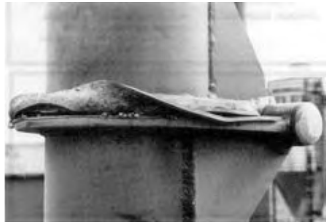
FIGURE 16. Seal Failure on Folding Discharge Boom.
