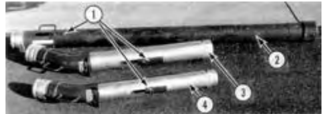
FIGURE 3. Intake Nozzles: (1) Adjustable Slide, (2) 5 in (125 mm) Diameter Steel Nozzle, (3) 5 in (125 mm) Diameter Aluminium Nozzle, (4) 4 in (100 mm) Diameter Aluminium Nozzle.
