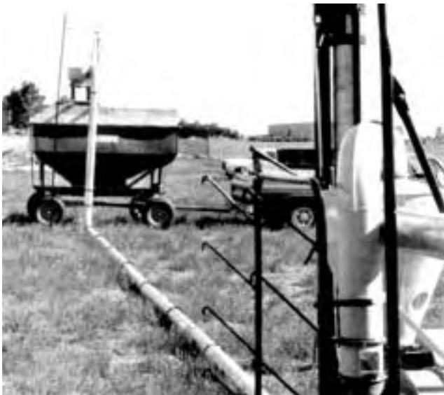
FIGURE 9. Increased Discharge Pipe Length.
