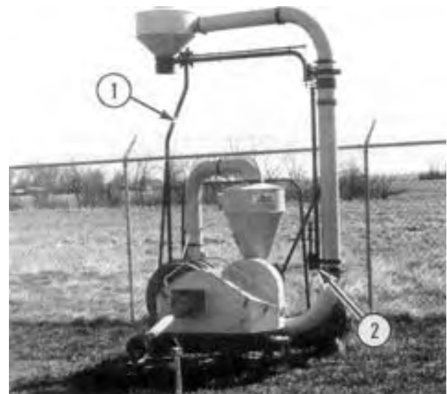
FIGURE 5. Kongskilde SUC 500 TR2 in Transport Position: (1) Support Bar, (2) Jack Assembly.
