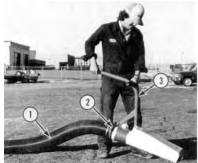
FIGURE 4. Position of Intake Nozzle to Clean Bin Floor Completely: (1) Flexible Vinyl Hose, (2) Clamp, (3) Detachable Handle.
