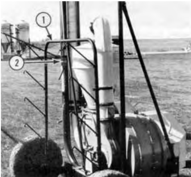
FIGURE 6. (1) Frame for Holding Pipe, (2) Locking Brake.
