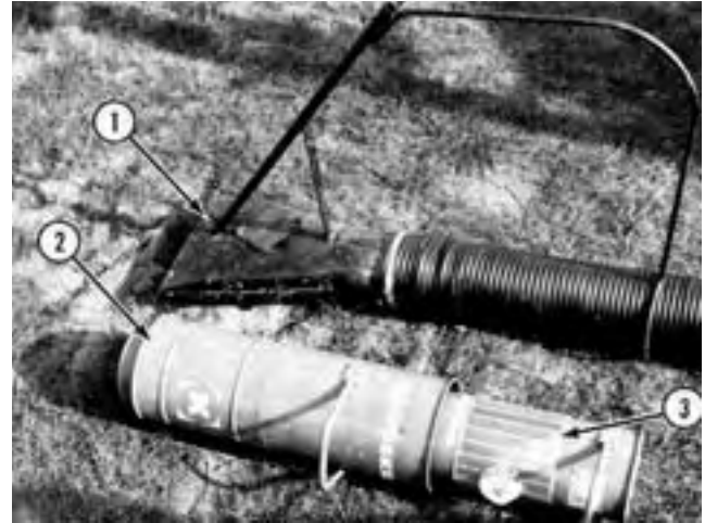
FIGURE 3. Intake Nozzles: (1) Flat Nozzle, (2) Round Nozzle, (3) Adjustable Sleeve.
