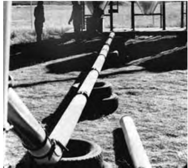
FIGURE 10. Increased Intake Pipe Length.
