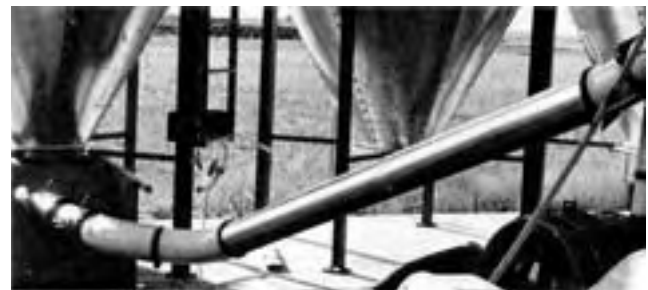
FIGURE 12. Rigid Intake Pipe Assembly.
