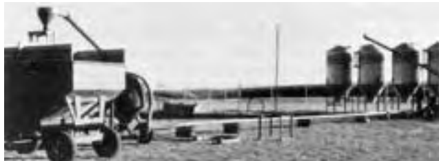
FIGURE 9. Increased Intake Pipe Length.
