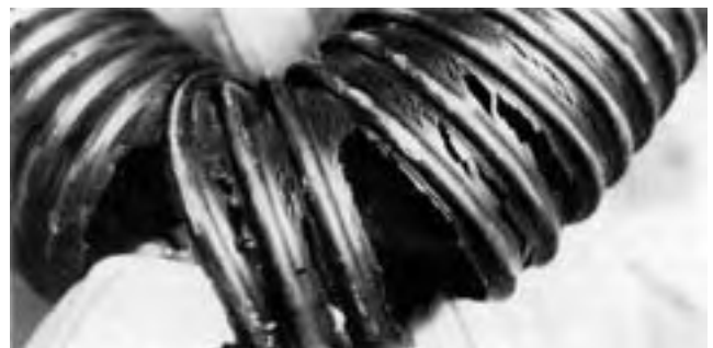
FIGURE 14. Failure of Polyurethane Hose due to Weathering.
