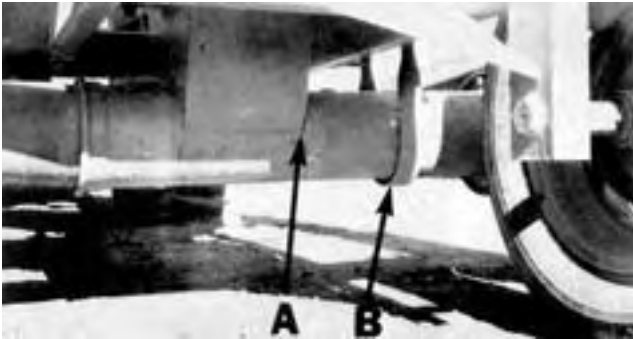
FIGURE 17. Cracked Discharge Tube: (A) Crack, (B) Supporting Brace.
