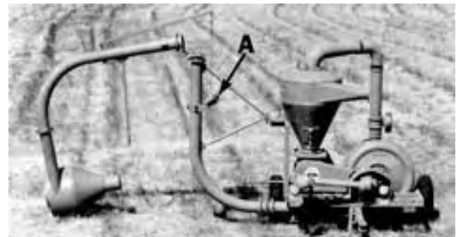
FIGURE 3. Cyclone Resting on Ground for Convenient Attaching: (A) Winch.
