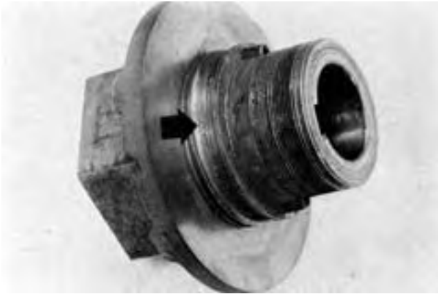
FIGURE 16. Worn Rotary Air Lock Hub.
