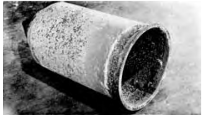
FIGURE 14. Separator Cyclone Screen Plugged with Fertilizer.
