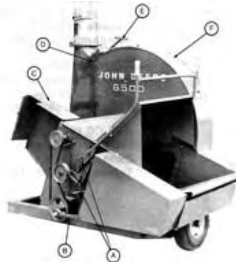
FIGURE 2. Blower (with hinged drive shield open): (A) Drive Belt Tension Adjustment, (B) Rocker Connecting Link, (C) Shield, (D) Band Guides, (E) Band Tightener, (F) Housing Band.
