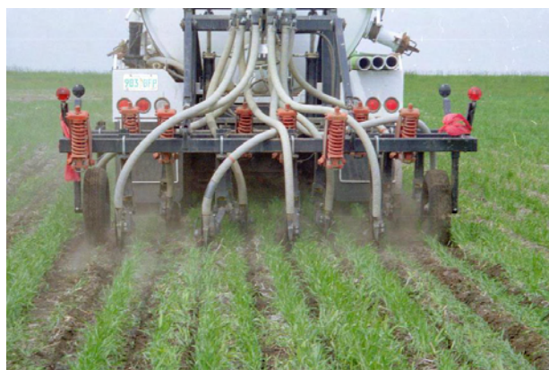
Figure 2. Soil disturbance from coulters.
