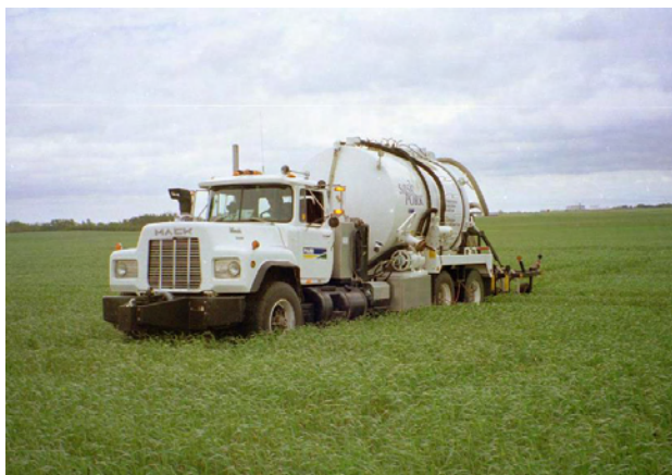
Figure 1. PAMI manure truck with coulters injectors.
