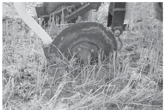
PAMI/Bourgault Low Disturbance Manure Injection Opener.
