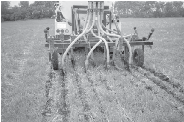
Low disturbance post-emergent injection of swine manure.
