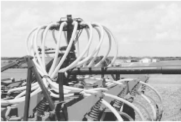
A sixteen port manifold distribution system was mounted on a Flexi-Coil 820 chisel plow with 16 openers placed at 12-inch (300 mm) row spacings.
