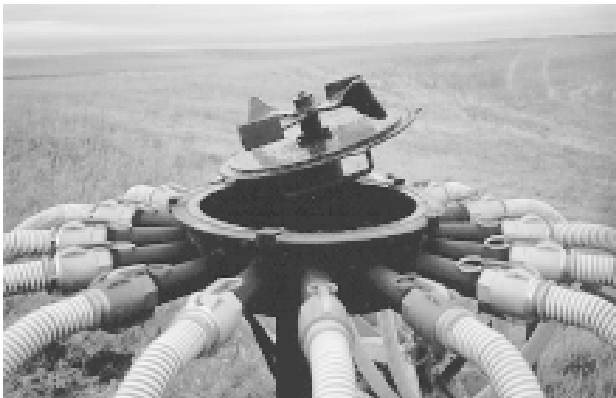
The slurry distribution manifold has a hydraulically powered, rotary cutting/distribution system.
