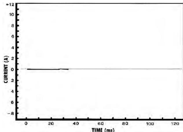
FIGURE 6. Current Delivered to a Normally-Grounded Cow Touching a 16 km Fence. Well-Insulated Fence.
