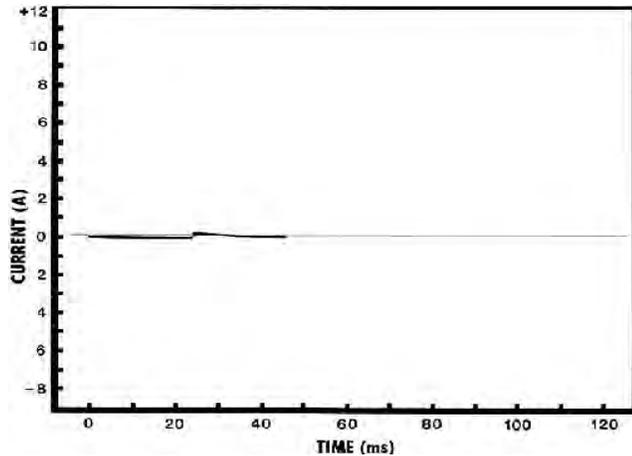
FIGURE 4. Current Delivered to a Well-Grounded Cow Touching a 16 km Well-Insulated
