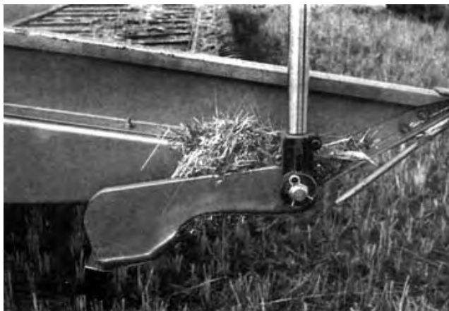
FIGURE 12. Material Build-up at the Right End of the Cutterbar.
