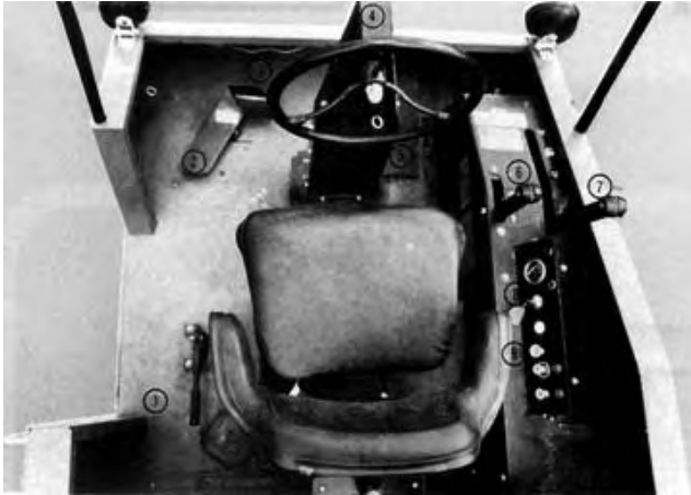
FIGURE 1. Operator's Platform. (1) Parking brake lever, (2) Header hydraulic control pedal, (3) Steering wheel, (4) Steering column and variable speed control, (5) Reel control pedal, (6) Throttle, (7) Header control lever, (8) Ignition switch, (9) Choke.
