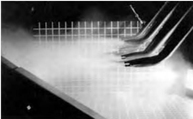
FIGURE 4. Deeper Air Blast with "Double Drop Tubes".
