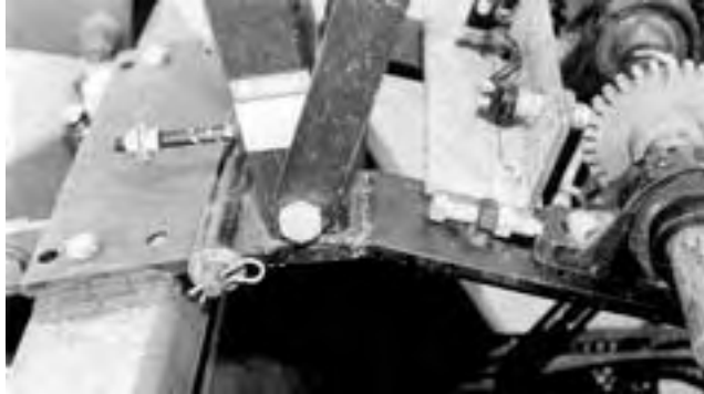
FIGURE 10. Weld Failure on Fan Mounting Bracket.
