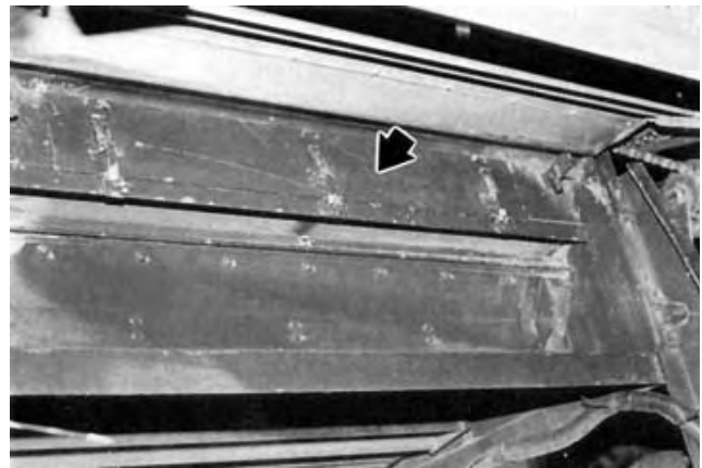
FIGURE 6. Stone Trap Clean-Out Door.
