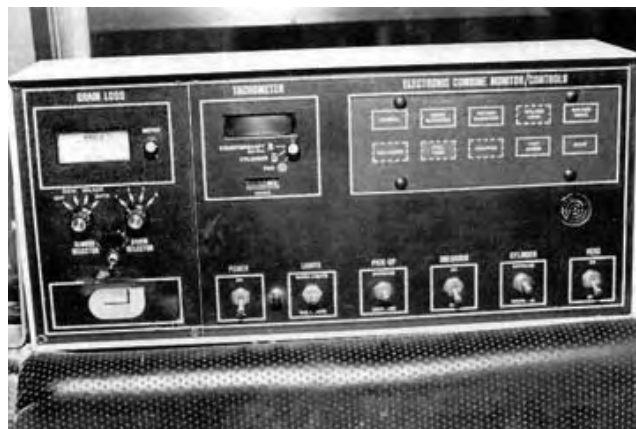
FIGURE 2. Electric Monitor/Control Box.
