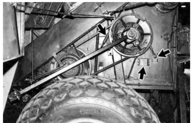
FIGURE 10. Concave Levelling and Inspection.
