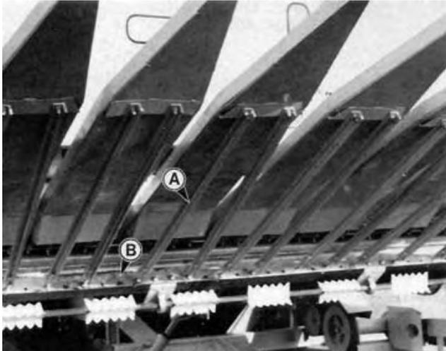
FIGURE 2. Seed Pan Supports: (A) Braces, (B) Support Bracket.
