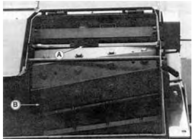
FIGURE 7. Cutterhead Assembly: (A) Knife Sharpener, (B) Knife.
