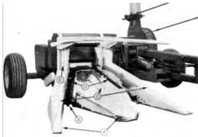
FIGURE 3. Two-Row Row Crop Head: (A) Divider Noses, (B) Oscillating Knife, (C) Nose Adjusting Straps, (D) Gathering Belts, (E) Gatherer Feedroll.
