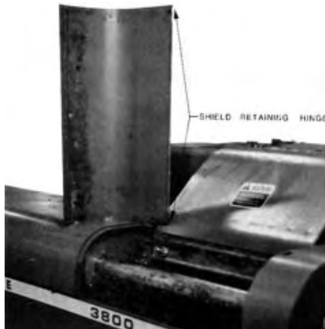
FIGURE 7. Fan Drive Shaft Shield.
