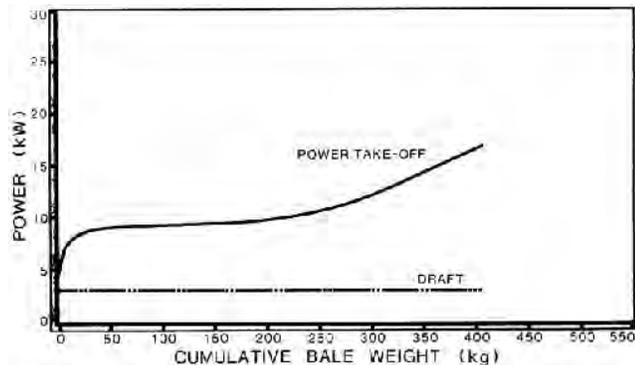
FIGURE 4. Power Consumption During Bale Formation in Alfalfa.
