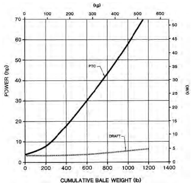
FIGURE 6. Power Consumption During Bale Formation in Alfalfa.
