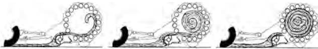
FIGURE 5. Stages of Bale Formation: (Left) Starting Bale, (Centre) Partially Completed Bale, (Right) Completed Bale.
