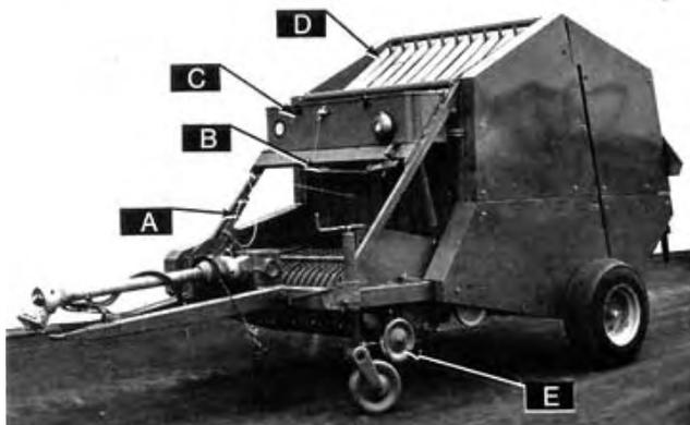
Figure 2. Front View of McKee 1500 Round Baler. Identification of components: (A) Pickup Transport Lever, (B) Twine Mechanism, (C) Twine Box, (D) Forming Belts, (E) Gauge Wheel.
