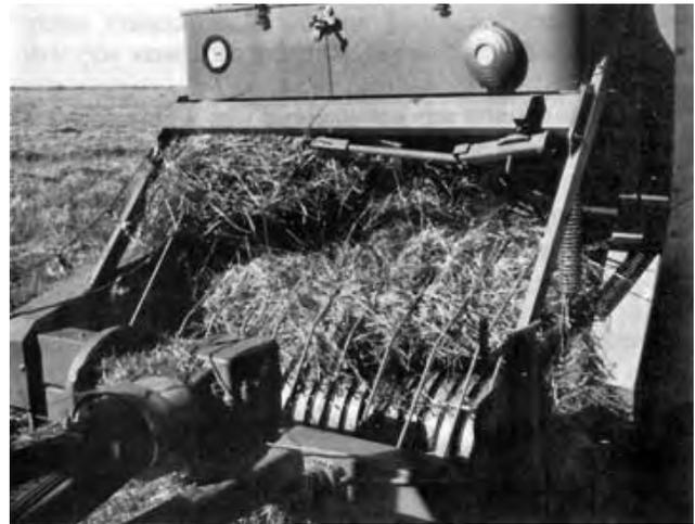
**Figure 7.** Plugging in Heavy Windrows Due to Excessive Lift of Compression Bars.
