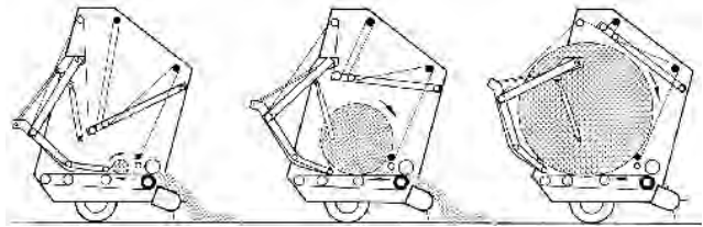
Figure 7. Stages of Bale Formation: (Left) Bale Core, (Centre) Half-Completed Bale, (Right) Completed Bale.
