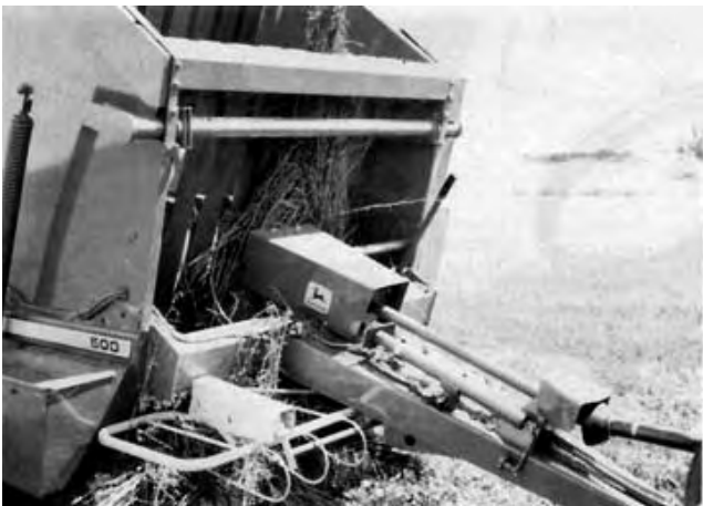
Figure 9. Plugging in Sweet Clover Before Compression Roll Modification.
