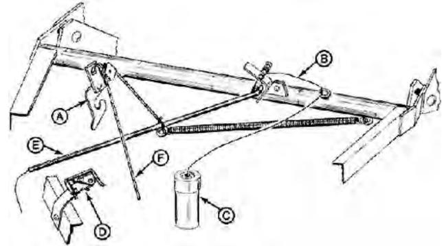
twine cutter assembly, (E) twine tube, (F) rope.
