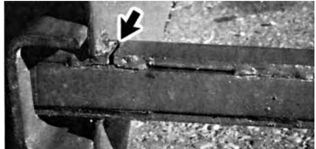
FIGURE 12. Failure of Bale Chute Frame Welds.
