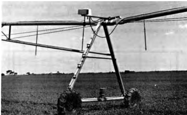
FIGURE 14. Lockwood Centre Pivot Support Tower.
