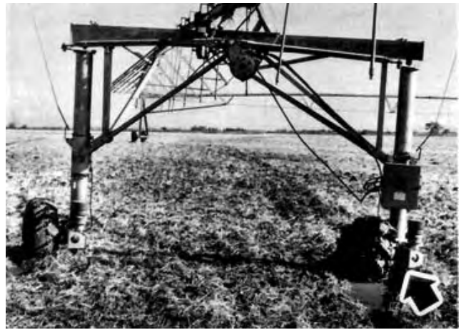
FIGURE 19. Broken Flexspan Corner Attachment Tower Axle.
