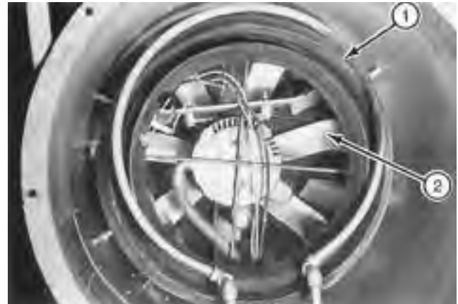
FIGURE 7. Fan Housing: (1) Burner, (2) Fan.
