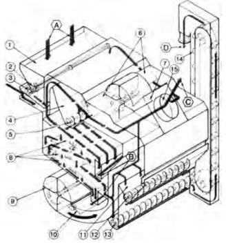
FIGURE 1. Forever 42 Dustless Grain and Grass Seed Cleaner, (A) Uncleaned Grain, (B) Screenings, (C) Dust and Chaff, (O) Clean Grain (1) Hopper, (2) Agitator, (3) Feed Roller, (4) Suction Settling Chamber, (5) Suction Auger (6) Suction Air Valve, (7) Suction Fan, (8) Screens (9) Blower Fan, (10) Blower Fan Control, (11) Blower Settling Chamber, (12) Blower Auger (13), Clean Grain Auger, (14) Bucket Elevator, (15) Dust Outlet.
