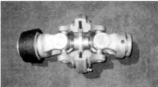
Figure 5. A Constant Velocity joint's driving members are steel balls constrained in curved grooves between the forks of the joint (photo at left). These joints are also called Double Cardan joints. This design operates efficiently up to a 80° deviation from a straight line (illustration at right).
