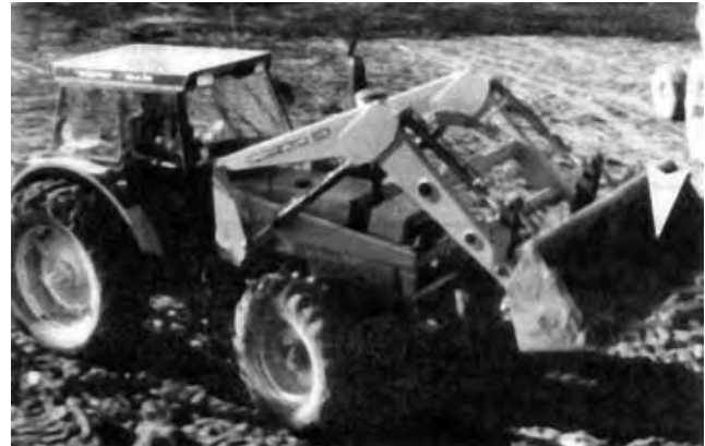
FIGURE 3. Damp Material Adhering to Bucket Walls.
