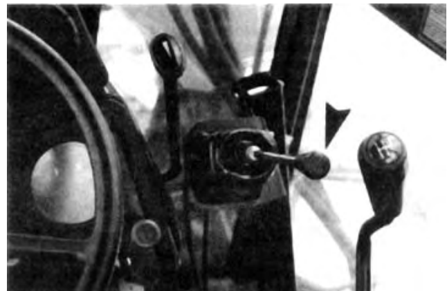
FIGURE 4. Single Lever "Joystick" Control.
