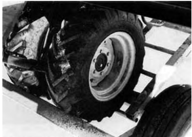
FIGURE 2. Drive Wheels Seated in Cradle.
