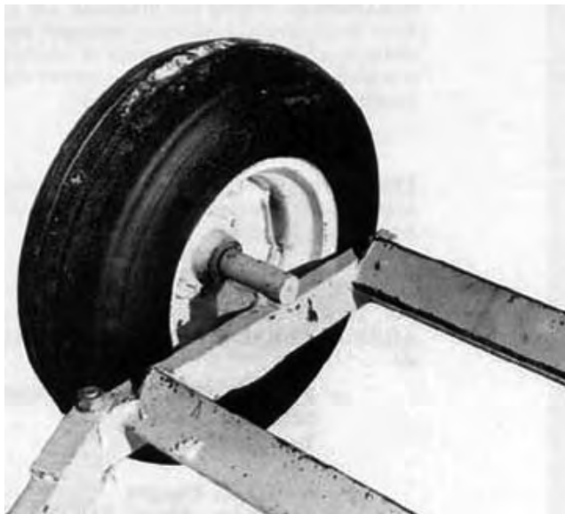
FIGURE 3. Laurier Transporter with Frame Inverted to Reduce Transport Height.
