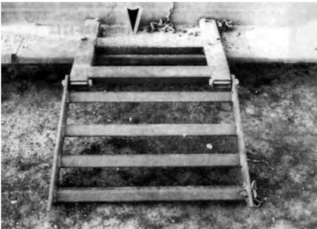
FIGURE 3. Windrower Loading Ramps Showing Spacer Added to Increase Header Clearance.
