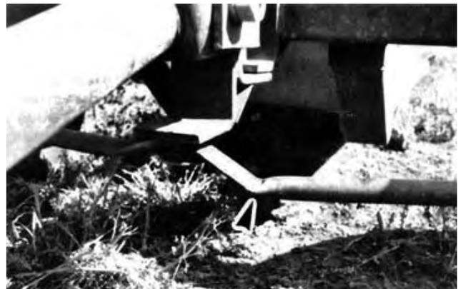
FIGURE 5. Bent Steering Tie Rod.
