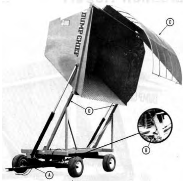
FIGURE 1. 706W Dump Chief: (A) Telescoping Tongue, (B) Mechanical Bolster Stabilizers, (C) Swing-Away Roof, (D) Extending Columns.
