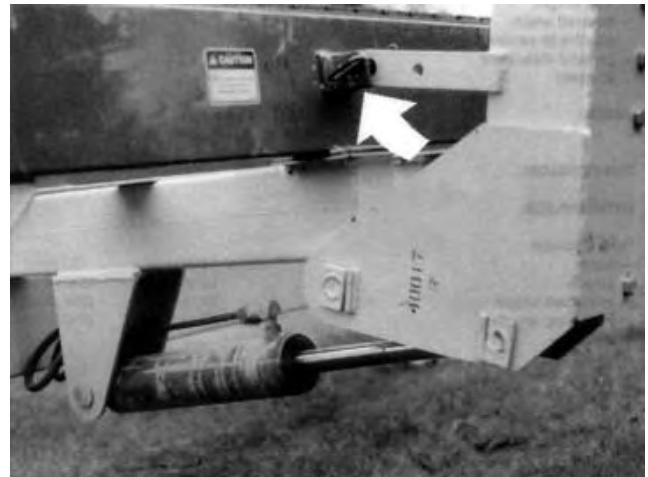
FIGURE 4. Lift Arm Safety Lock Pin.
