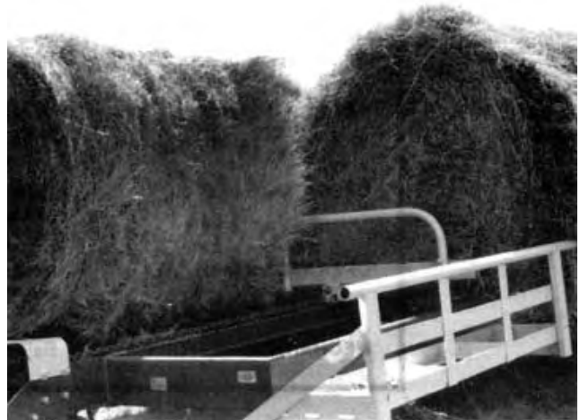
FIGURE 4. Bale Drag Trapped Between Bales.
