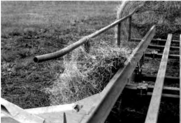
FIGURE 5. Twine Snagged by Optional Right Hand Side Rail.
