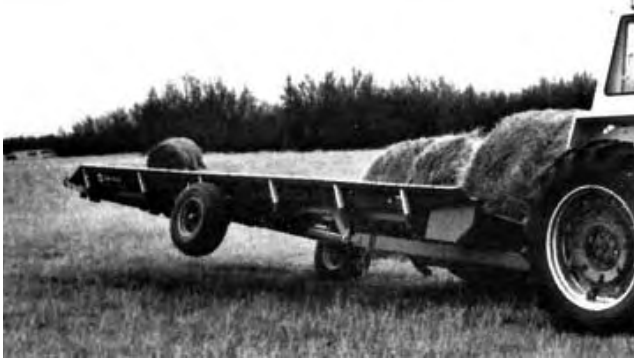
Figure 3. Sideways Tipping of the Bale-rustler when the First Bale Loaded Weighs More than 680 kg (1500 lb)
