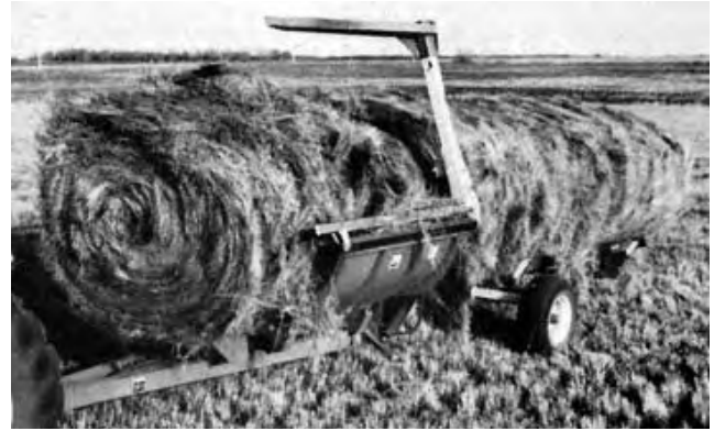
Figure 5. Fully Loaded Bale-rustler. Bales are Rotated During Loading Leaving the Weathered Side Down.
