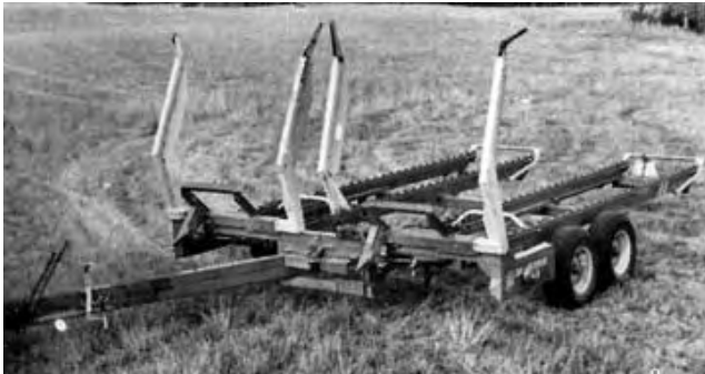
Figure 2. B & K 815 With the Tongue Positioned for Loading the Left Bed.
