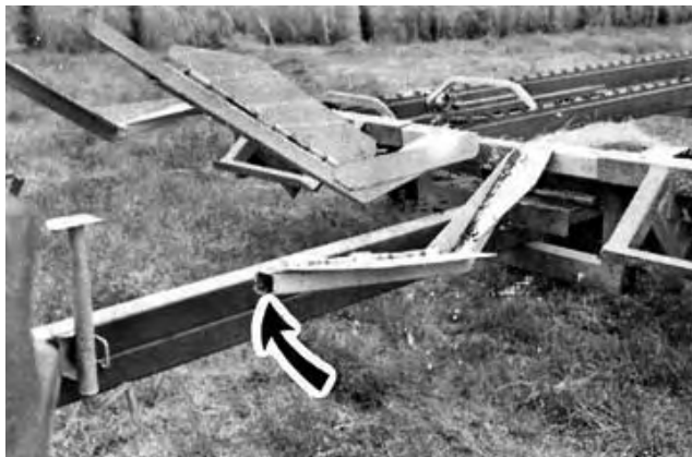
Figure 10. Broken Tip on Pickup Fork Tine.
