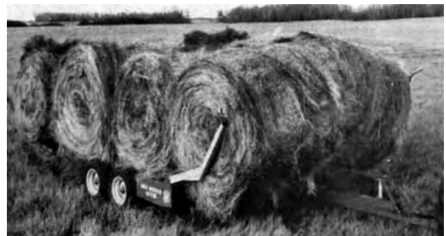
Figure 5. B & K 815 Fully Loaded in Transport Position.
