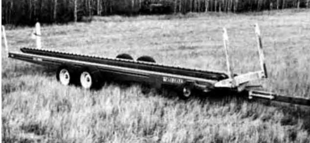
Figure 1. Farmhand F126-B in Transport Position.
