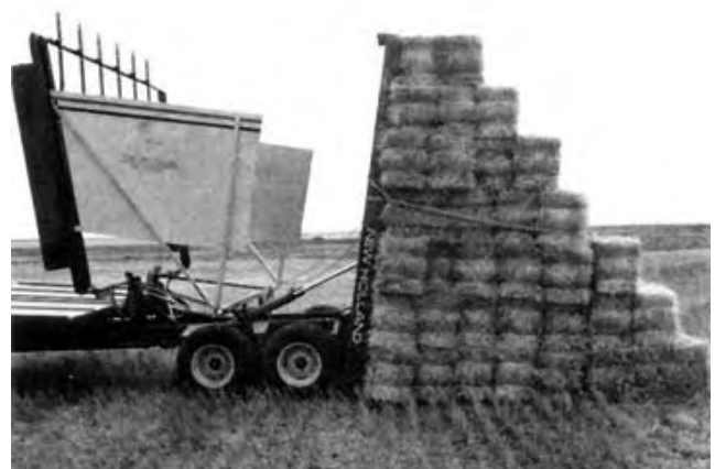
FIGURE 5. Suitable Backstop Formed by Rearranging a Full Load by Hand.
