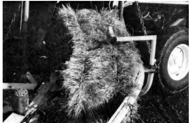
FIGURE 7. Bending of Bale in the Loader.
