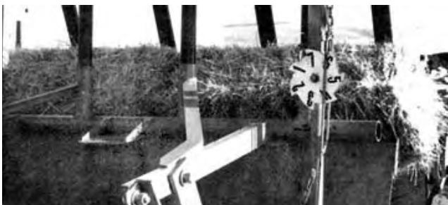
FIGURE 10. First Lift of Bales Slipped Sideways in Rough Fields.
