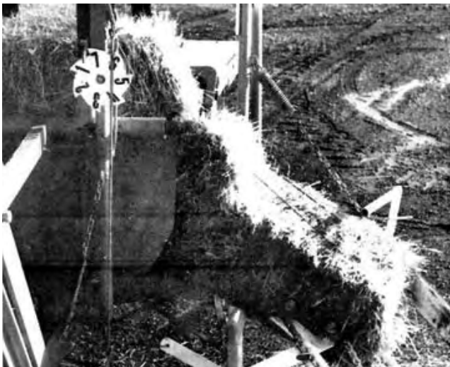
FIGURE 9. Loose Bale Wedged on Bale Chamber Side.
