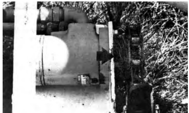
FIGURE 8. Twine Build-up on Loader Drive Sprocket.
