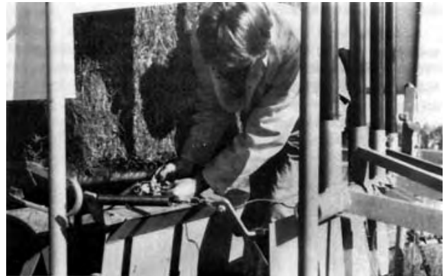
FIGURE 15. Reaching Under Partially Raised Load Deck to Initiate a Tie.
