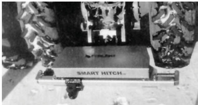
Figure 13. The Smart Hitch Guidance System steers the cultivator from the rear of the tractor. Photo Source: Smart Hitch photo, used by permission.
