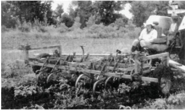
Figure 7. Operator Steered Cultivators are safer if the operator is positioned at the rear of the cultivator, facing direction of travel.
