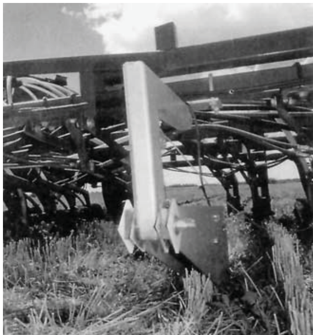
Figure 14. The Smart Hitch Guidance System mates to a steering mechanism on the cultivator. Photo Source. Western Producer/ Michael Raine. Used by permission.
