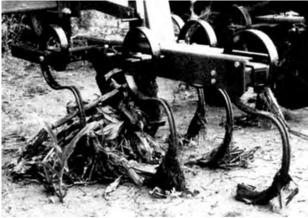
FIGURE 5. Plugged gang due to gauge wheel interference.
