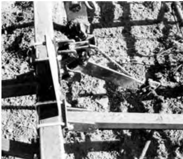
FIGURE 9. Rod Shank in Tripped Position.
