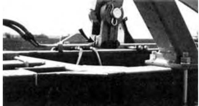
FIGURE 12. Hydraulic Cylinder Yoke Failure.
