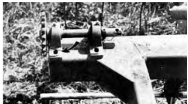
FIGURE 14. Rod Drive Pillow Block Failure.
