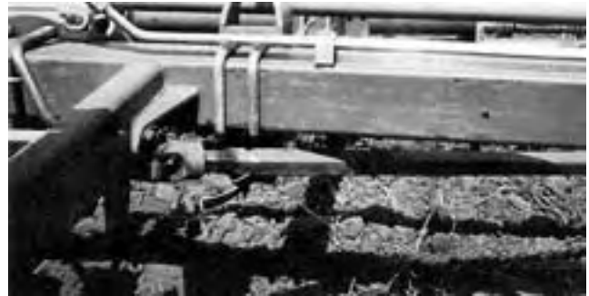
FIGURE 13. Interference of the Frame with the Rod Drive Shaft.
