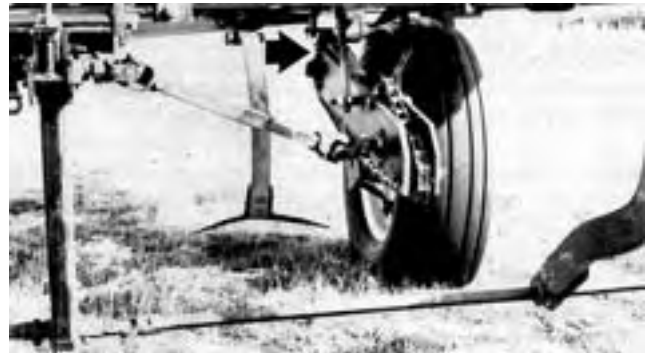
FIGURE 8. Centre Drive Assembly in Transport Position.
