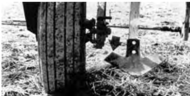
FIGURE 10. Sweep Wing Cut Off to Prevent Centre Rod Drive Assembly Interference.
