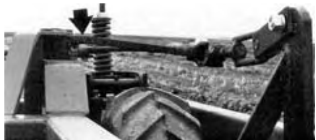
FIGURE 15. Bent Depth Control Pivot Arm.
