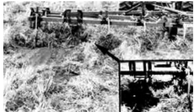
FIGURE 4. Plugging at the Wing Section Drive Shafts.
