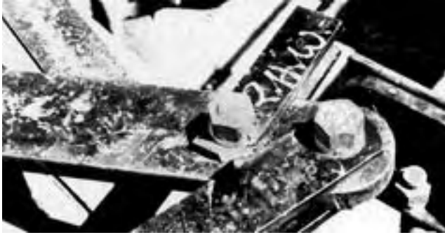
FIGURE 16. Corner of Right Depth Control Rod Clevis Cut Off.
