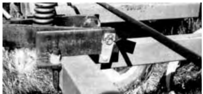
FIGURE 14. Weld Failure on a Rod Shank Swivel Locking Bar.
