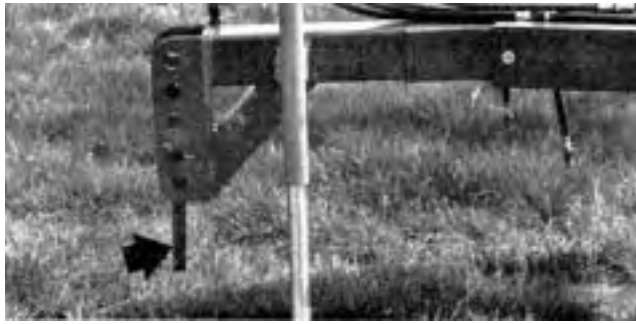
FIGURE 9. Hitch Link in Vertical Position.
