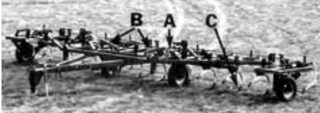
FIGURE 1. Edwards GN-R78-436: (A) Master Cylinder, (B) Wing Lift Cylinders, (C) Cultivator Shanks.
