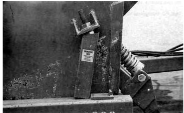
FIGURE 6. Improperly Positioned Transport Locks.
