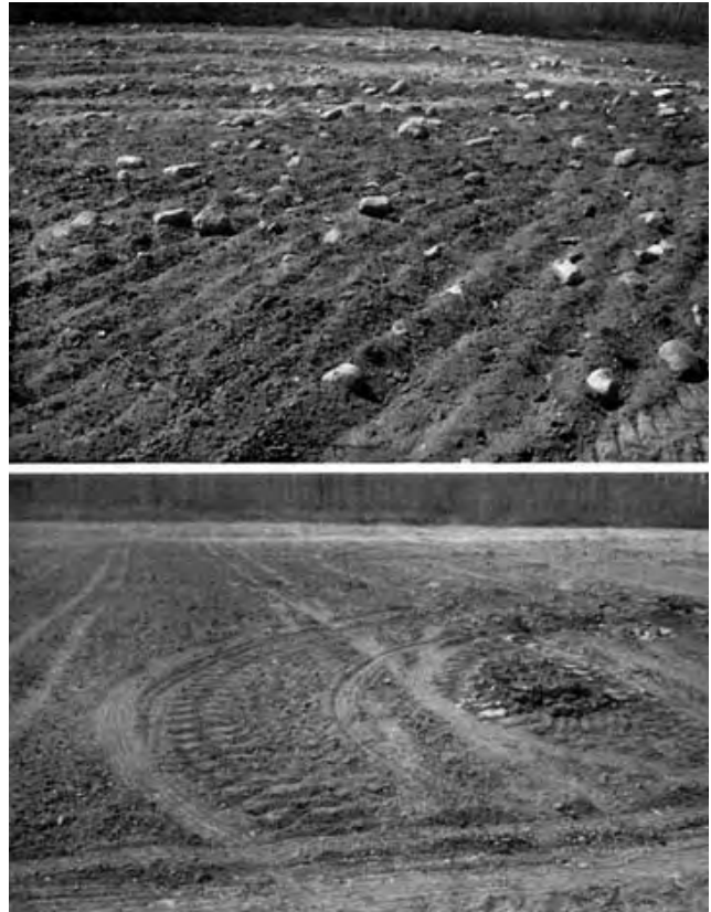
FIGURE 4. Performance in Large Rocks: (Top: Before Picking, Bottom: After One Pass with Picker).
