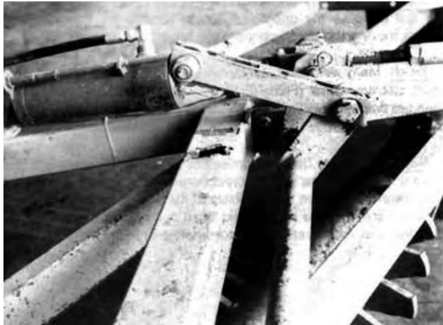
FIGURE 4. Damaged Transport Lock Bracket Caused by Inadvertent Movement of Depth Control Cylinder with the Lock in Place.
