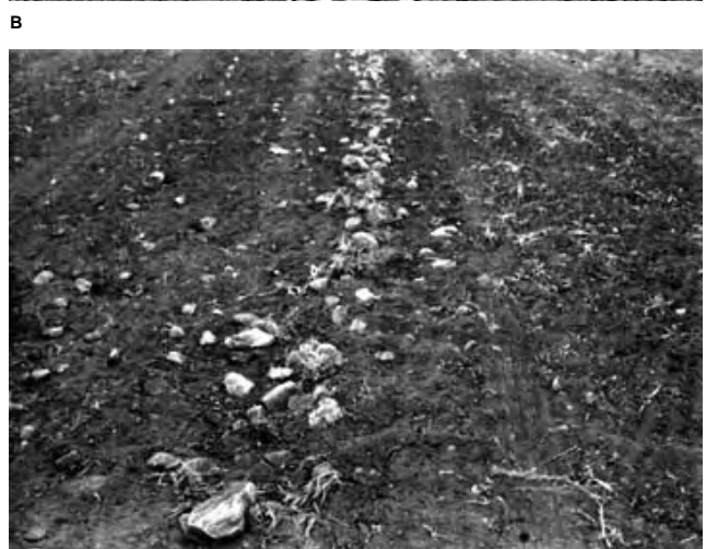
FIGURE 2. Typical Performance in a Field with Medium Rock Concentration: (A) Before Windrowing, (B) Windrowed at 5 km/h, (C) Windrowed at 7 km/h.
