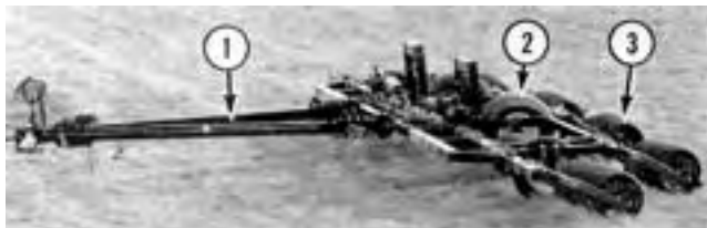
FIGURE 1. Bourgault WTP 36-40 Wing Type Packer: 1) Telescoping Hitch, 2) Transport Wheels and 3) 1.5 in (38 mm) Steel Coil Packers.
