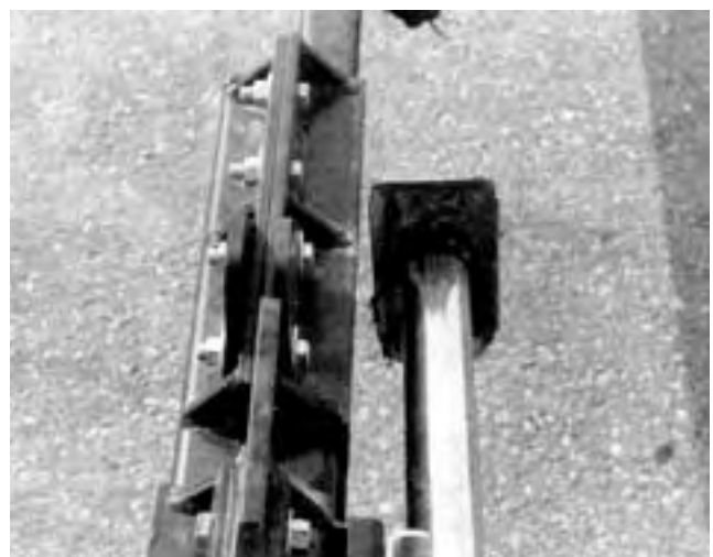
FIGURE 6. Poor alignment of hitch extension brackets.
