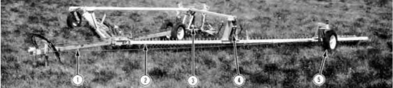
FIGURE 1. Phoenix Rotary Harrow Model HT140: 1) Hitch Frame, 2) Wing Frame, 3) Transport Motor Drive Location, 4) Tine Lift Cylinders, 5) Wing Wheels.
