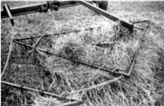
FIGURE 3. Harrow Plugging in Damp Straw.
