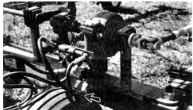
FIGURE 8. Hoses Rubbing on the Tire.
